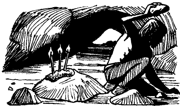
▲ Working in a Bronze Age copper mine. Extra light is provided by burning pine chips.
